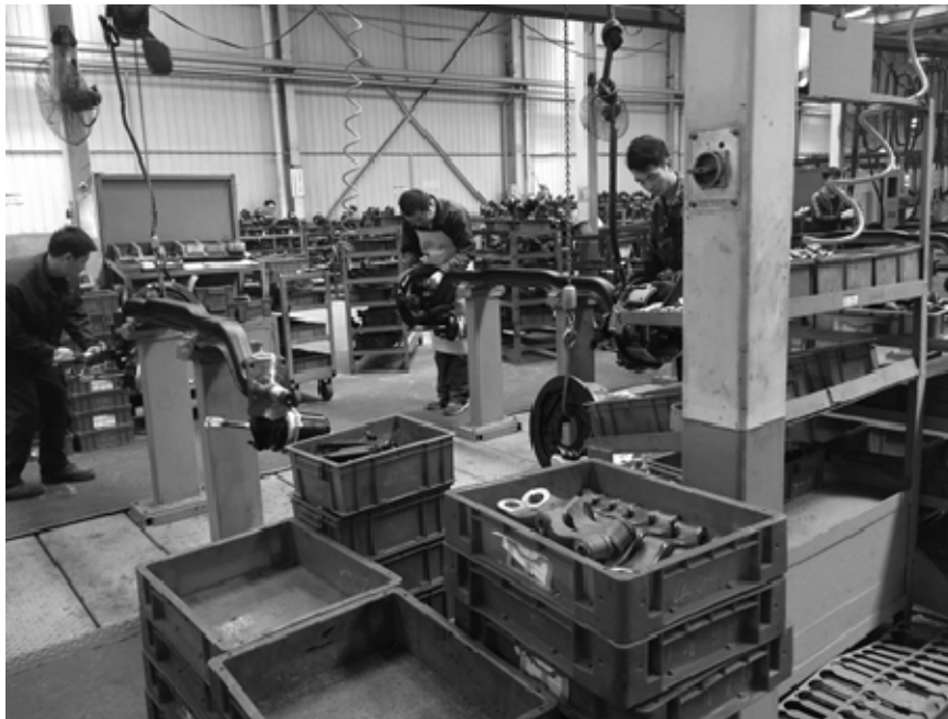
Figure 5: assembly of axles according to the continuous-production principle
